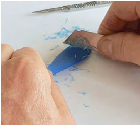
Working from the hub to the tips, scrape the blades evenly checking for balance as you go.
