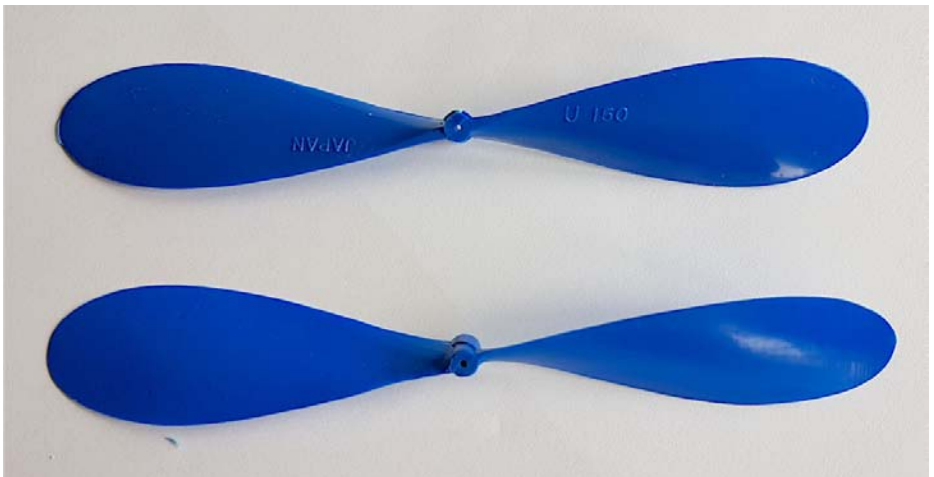
Working from the hub to the tips, scrape the blades evenly checking for balance as you go.
